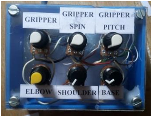
Fig. 5: The potentiometer control section
