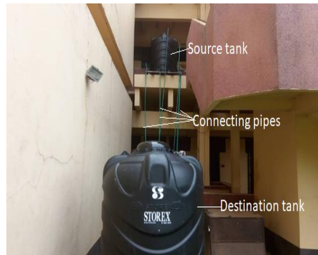
Fig. 6: Experimental rig for water flow rate and leakage experiment
