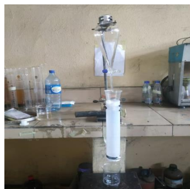
Fig.1: Batch Adsorption Column set-up for the experiment
