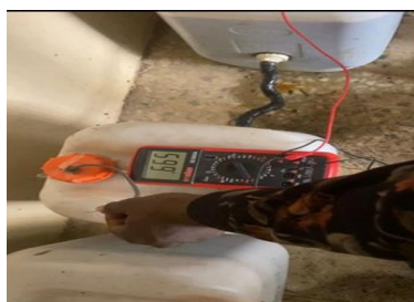
Fig. 4: Evaluation of electricity generated from one of the MFC set-ups
